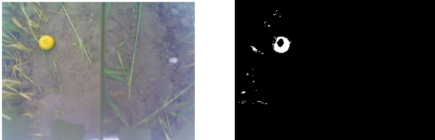
Figure 16: Original image (left), thresholded image (right)
