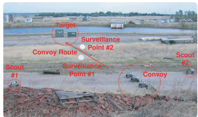
FIGURE 19 A target-assessment mission. A team of six robots is commanded to approach a target and relay camera images that allow the user to assess the target's condition. Initially, two scout robots inspect the path to ensure its safety. The four remaining robots then proceed in formation to the target and send back images.
