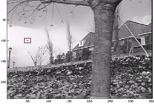
Fig. 6. Low texture region, gradients with small magnitude, small eigenvalue.
