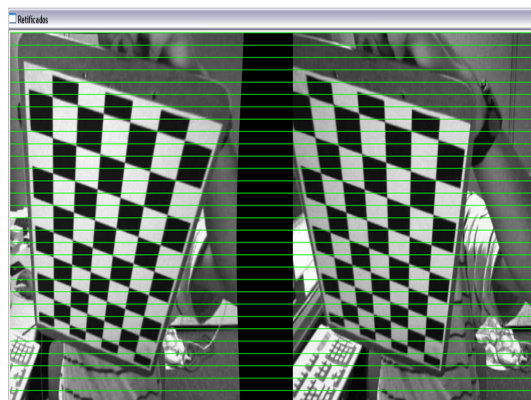
Figure 6. Rectified Images using Hartley's algorithm.
