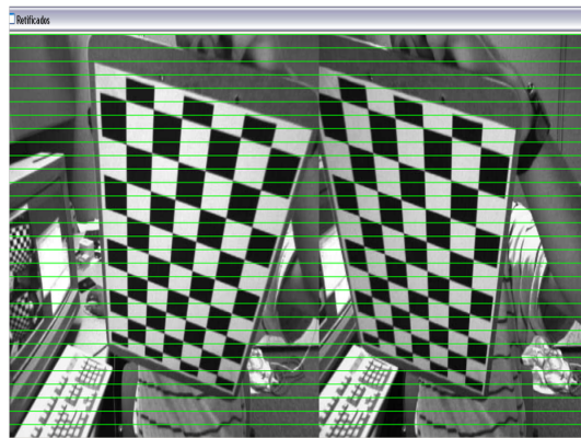
Figure 5. Rectified Images using Bouguet's algorithm.
