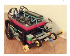
HandyBug design is equipped with a **bend** sensor "outrigger," enabling it to detect its distance from the wall. The closer to the wall, more the sensor is flexed. This increases its resistance, and a greater value is detected by *HandyBug*'s sensor circuitry.
