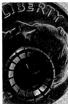
Figure 7.3. This 8 millimeter (mm) diameter piezoelectric ultrasonic motor, built at the MIT Mobile Robot Lab, is composed of two pieces: the stator and the rotor. The stator , shown on the left, is a steel ring with piezoceramics bonded onto the bottom that causes a wave to travel around the ring. The top piece, the rotor , is made of brass and, when pressed against the stator, is dragged along and spins. The stator with a rotor on top is illustrated on the right.
