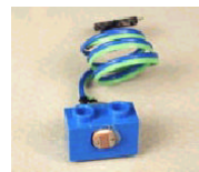
Photocell Sensors Mounted on LEGO Technic Beam
