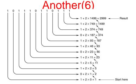
Conversion of the binary number 101110110111 to decimal by successive doubling, starting at the bottom. Each line is formed by doubling the one below it and adding the corresponding bit. For example, 749 is twice
