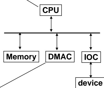
CPU sends a starting address, direction, and length count to DMAC. Then issues "start".
